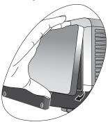
4. Loosen the screws that hold the lamp to the projector. If the screws are not loosened completely, they could injure your fingers. It is strongly recommended that you use a magnetic-head screwdriver to retain the screw should it come loose.
